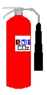
A CO<sub>2</sub> may be ineffective in extinguishing a Class A fire because it may not be able to displace enough oxygen to successfully put the fire out.
