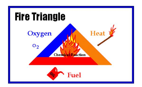
APW's extinguish fire by taking away the "heat" element of the Fire Triangle.
