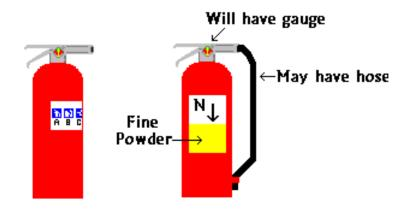
The "ABC" fire extinguishers are filled with a fine yellow powder. The greatest portion of this powder is composed of monoammonium phosphate. The extinguishers are pressurized with nitrogen.
