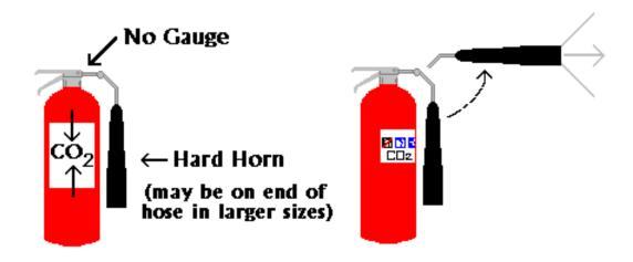
The pressure in a CO<sub>2</sub> extinguishe r is so great, bits of dry ice may shoot out of the horn!
