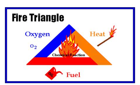
Dry chemical extinguishers put out fire by coating the fuel with a thin layer of powder. This separates the fuel from the oxygen in the air.
