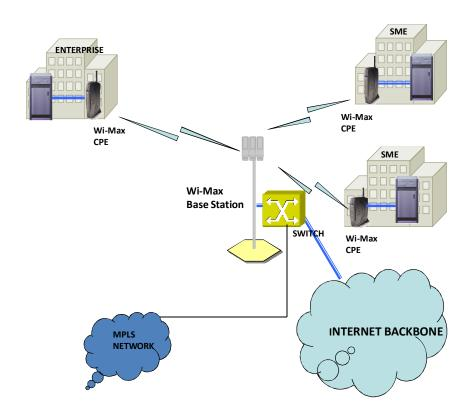
Wi-MAX for providing MPLS-VPN connectivity
