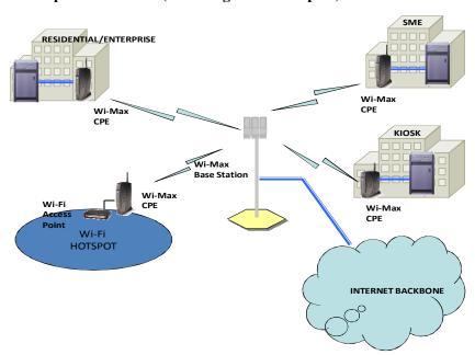
Wi-MAX for providing Wireless Broadband connection for residential / enterprise customers (including Wi-Fi hot spots)
